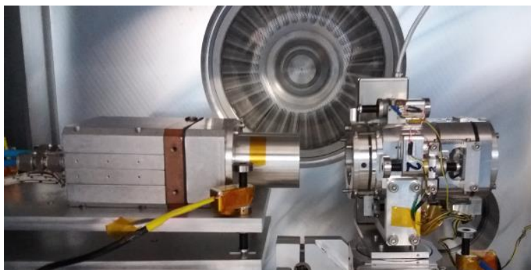
Fig. 1: Picture of the high NA EUV wavefront sensor (left) in front of a EUV Schwarzschild objective.
