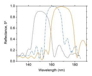
Narrowband FUV coatings can be prepared with all-dielectric multilayers (MLs) based on two fluorides. The relatively higher expansion coefficient of fluorides in comparison with common substrates such as fused silica (FS) or Zerodur<sup>®</sup>, results in large tensile stress for coatings deposited on a heated substrate and later cooled down to room temperature. Such stress may result in coating cracking and/or delamination in a process that grows with the number of layers.
