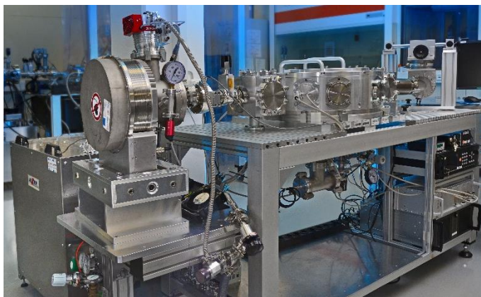
Fig. 1 Left: Photograph of the stand-alone EUV spectrometer. Right: Map of experimentally obtained reflectance data of a nanostructured sample serving as a basis for sample parameter reconstruction.
